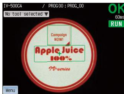
PASS Detection of sticker presence/absence by using position adjustment
