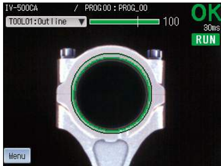
PASS Model type detection by internal diameter difference of metal part
