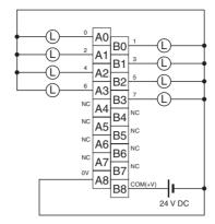
When wiring, pay careful attention to the polarity of the external power supply. The load may operate if the polarity is reversed.
