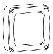
Banner's WLC90 Heavy Duty Lights are designed to operate in harsh environments and withstand washdown and spray from water as well as many chemicals including coolants and detergents. They are compact and bright, making them an excellent choice for machining centers and food processing equipment.
